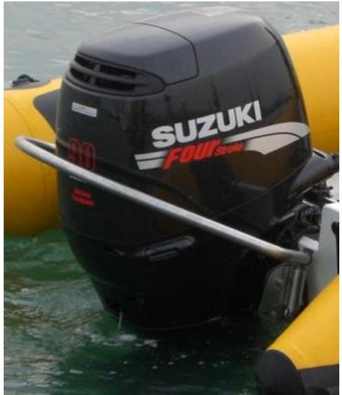
**Before setting the pre-trim" angle, trim the outboard motor fully down into its lowest position.**
