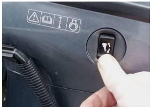
Assuming for instance a planing angle of 10 degrees, you may give the TurboSwing a "pre-trim" of 20-30 degrees, resulting in a 10-20 degree upward position in planing mode.
